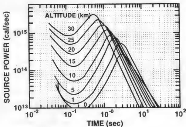
Figure 6.13. Effects of Altitude on Thermal Power for a 10-MT Burst.
